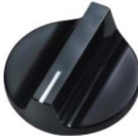
46011 Pointer knob with paint filled indicator line on top Material: NYLON Diameter: 33.2 mm Height: 17.4 mm
